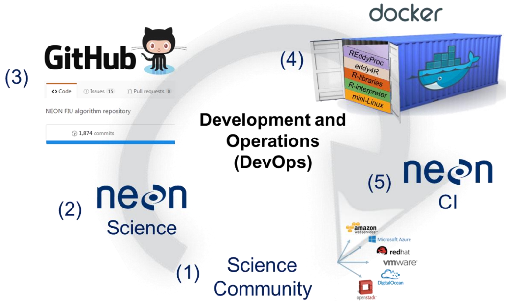
Figure 2. NEON’s DevOps framework consists of a periodic sequence: The science community contributes algorithms and best practices (1) which together with NEON Science (2) are compiled into eddy4R packages via the GitHub distributed version control system (3). NEON Science releases an eddy4R version from GitHub, which automatically builds an eddy4R-Docker image on DockerHub as specified in a “Dockerfile” (4). The eddy4R-Docker image is immediately available for deployment by NEON Cyberinfrastructure (CI; 5), the Science Community (1) and NEON Science (2) alike. This DevOps cycle can be repeated for continuous development and integration of requests and future methodological improvements, resulting in the next release.
