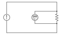
Figure 1. Four-wire measurement for PRT.
