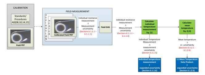
Figure 2: Displays the data flow and associated uncertainties of individual temperature measurements and L1 mean SAAT DPs. A detailed explanation of the PRT calibration procedures, please refer to AD[08,10,14].
