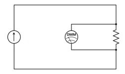
Figure 1. Four-wire measurement for PRT.
