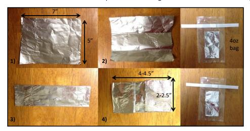
Figure 3 Steps to create foil packets: 1) cut a  $\sim 7''$  x 5" rectangle of foil, 2) mark lines to fold into thirds, 3) fold into thirds along the longer edge, 4) fold in the ends to close the packet. Keep a 4oz Whirl-pak bag nearby to make sure packets will fit.
