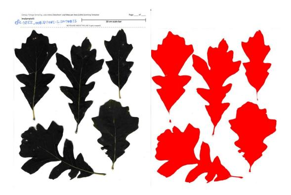
Figure 9 Left: Example of a good quality scanned image of foliage. Right: Image after processing in ImageJ
