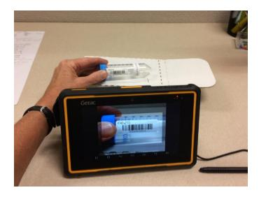
Figure 7. Barcode label scanning.
