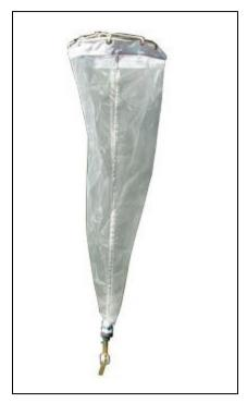
**Figure 9.** Zooplankton tow net with bottom tubing and clamp.
