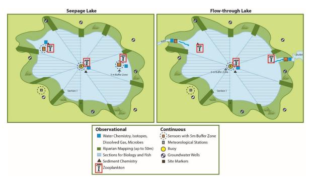
**Figure 3.** A generic lake site layout with zooplankton sampling locations. Seepage lakes have no true inlet or outlet stream. In flow-through streams, inlet and outlet infrastructure are located in the inlet or outlet stream channel.
