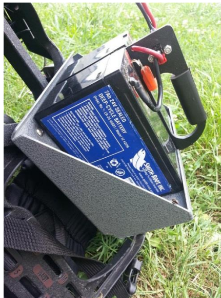
Figure 6. Battery location and secure placement in the backpack electrofishing frame
