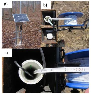
**Figure 11** (a) Standard groundwater well at a NEON site (b) Water-level tape attached to outer well casing. (c) Reading the depth to water from the water-level tape. The tapes are marked in "meters" with each foot increment marked in red. Readings are taken at the top of the inner PVC casing.
