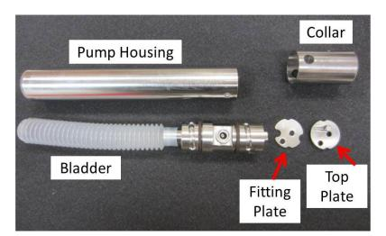
Figure 14. Components of the sampling pump
