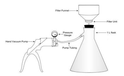
**Figure 23.** Filter apparatus set-up for particulates, using a) the vacuum pump and filter manifold, and b) the hand vacuum pump attached to the filter flask and filter funnel.
