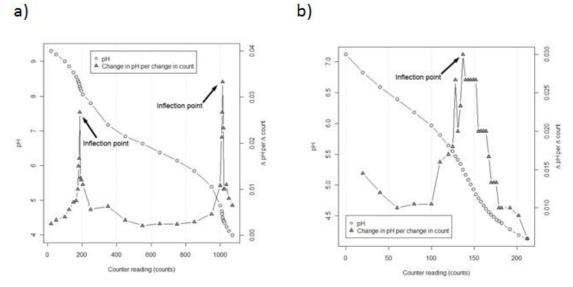
**Figure 28.** Example of inflection point titration using a digital titrator of a) a high alkalinity sample and b) a low alkalinity sample. Note difference in Y-axis scale. (Modified from USGS TWRI Book 9, Alkalinity, Version 3.0 7/2006).
