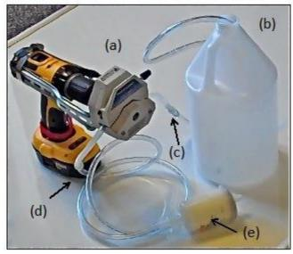
**Figure 22.** Pump and filter setup, including (a) a peristaltic sampling pump (modified from Woessner 2007), (b) a 4 L sample bottle, (c and d) tubing connectors to connect peristaltic and C-flex tubing, and (e) a capsule filter
