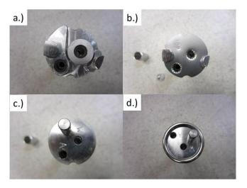
**Figure 13.** Assembly of the fitting plate at the top of the pump for holding the air and water lines. (a) Bare top of pump. (b) Fitting/grab plate added ("TOP" must face upwards). (c) Top plate added. (d) Collar added to lock parts (a-c) together.
