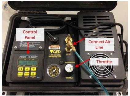
Figure 17. Attach blue air-line to controller
