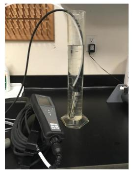
Figure 19. Groundwater Chemistry Collection cell using a 1000 mL graduated cylinder.
