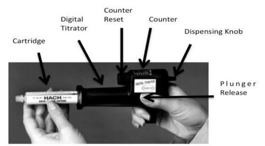
Figure 24. Inserting titrant cartridge into digital titrator. Photo from the Hach Digital titrator manual
