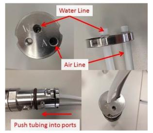
**Figure 15.** Attaching grey air-line and white water-lines to pump (top-right photo shows lines pushed through top plate and "teeth" of grab plate)
