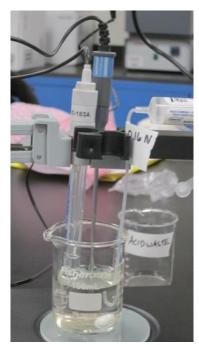
**Figure 27.** Image of titration set-up with digital titrator, stir bar, pH meter and temperature probe. Ensure nothing is touching the sides and bottom of the beaker or the stir bar
