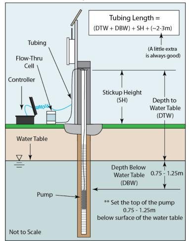
Figure 12. Cut tubing to the correct length.
