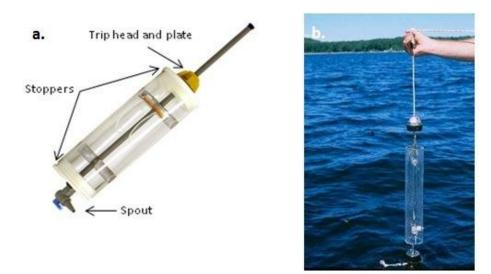
**Figure 10**. Illustration of Kemmerer sampler for water sampling (a). Illustration of how the Kemmerer is lowered into the water by holding the rope and messenger (b)
