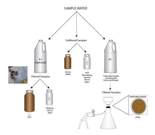
**Figure 5**. Flowchart of Water Chemistry Sample Collection and Filtration.  $\diamond$  Indicates 250 mL, wide-mouth sample bottles that remain at the Domain Support Facility for analysis. Letters in parenthesis indicate the codes that correspond to the chemistry labels (see Figure 6).
