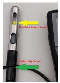
Figure 7. Picture of handheld meter showing location of sensors on probe.
