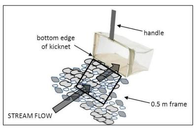
Figure 25. Example of modified kicknet setup.
