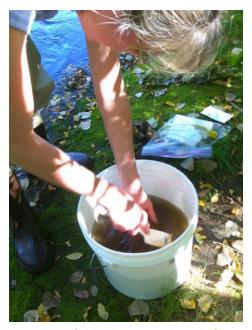
**Figure 18.** A field technician scrubs rocks from the Surber sample into the 3 gallon bucket
