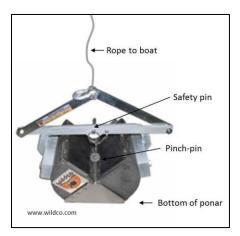
Figure 20. Example of a petite ponar setup
