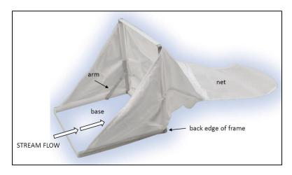
**Figure 14**. Diagram of Surber sampler set-up. The inside of the base is the sample area of the stream bottom (0.09 m2).
