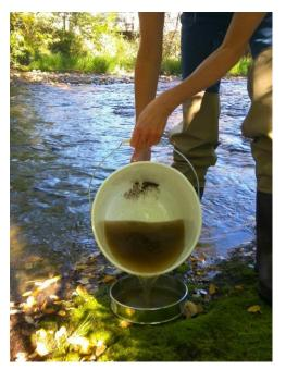
**Figure 31.** A field technician carefully pours water from the 3 gallon bucket into the sieve.
