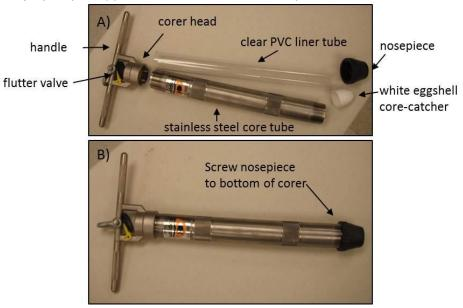
**Figure 23**. Hand-corer assembly: A) Disassembled corer. Use of the liner tube and core catcher are optional. B) Assembled corer. Note: the nosepiece may be stainless steel (not black Lexan as in photo) in some domains
