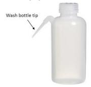
Figure 19. Removing the tip of the 500 mL wash bottle helps makes rinsing easier and increases water pressure. This tip pulls easily out of the main body of the wash bottle.
