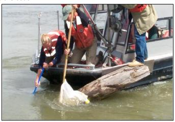
**Figure 22.** From Angradi et al. 2006, example of snag sampling in a large river. While the boat driver holds the boat in position, one technician holds the modified kicknet against the snag, while a second technician scrubs the snag with a long-handled deck brush.
