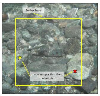
**Figure 17**. Cobble selection at Surber edges. The yellow square represents the bottom of the Surber sampler.
