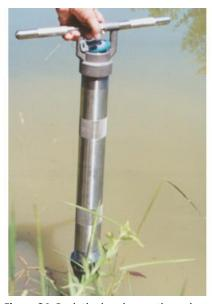
**Figure 24.** Push the hand corer through the water and into the sediments at a 90° angle
