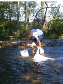
**Figure 16**. Hold the Surber net on the stream bottom, and keeps the bucket nearby for depositing rocks from the base of the Surber.
