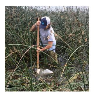
**Figure 29.** D-frame sweep technique in a littoral area; the D-frame net must remain submerged and close to the substrate throughout the entire sweep.
