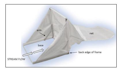
**Figure 15**. Diagram of Surber sampler set-up. The inside of the base is the sample area of the stream bottom (0.09 m2).
