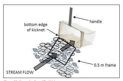
Figure 25. Example of modified kicknet setup.
