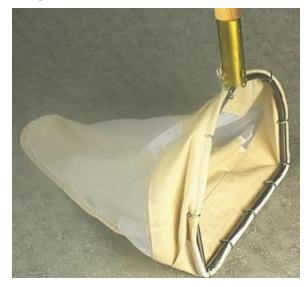
**Figure 28.** D-frame net, used for sweep samples in vegetation and silty habitats.
