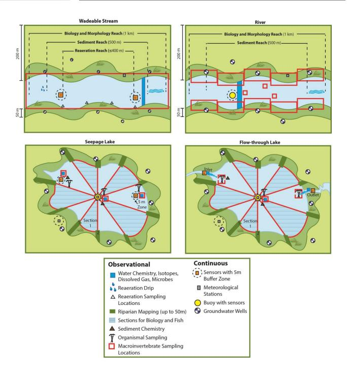
**Figure 10.** Generic site layouts with macroinvertebrate sampling locations in red. Seepage lakes have no true inlet or outlet stream. In flow-through streams, inlet and outlet infrastructure are located in the inlet or outlet stream channel.
