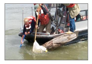
**Figure 22.** From Angradi et al. 2006, example of snag sampling in a large river. While the boat driver holds the boat in position, one person holds the modified kicknet against the snag, while a second scrubs the snag with a long-handled deck brush.
