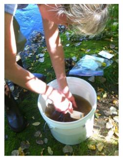
**Figure 18.** Scrub rocks from the Surber sample in the 3 gallon bucket
