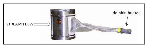
Figure 26. Hess sampler with collection net and dolphin bucket
