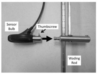
Figure 5. Velocity meter and the thumbscrew that attaches it to the wading rod
