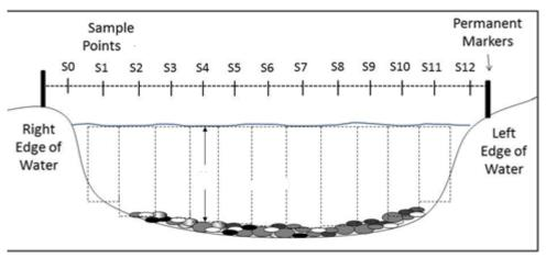
Figure 2. Example of an excellent distribution of measurement section
