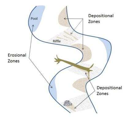
Figure 1. Examples of depositional zones in a wadeable stream.
