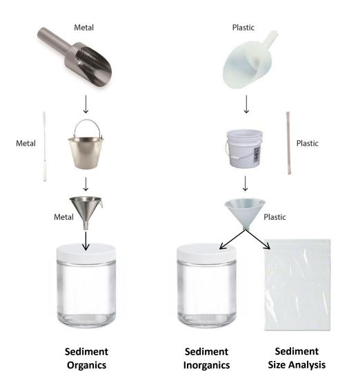
Figure 11. Sediment collection instruments by sample type
