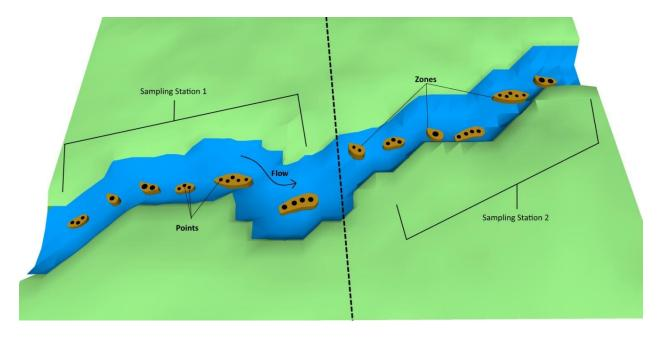
**Figure 3.** Identifying the location for sediment sampling in wadeable streams. The two sediment sampling stations should contain 5-10 depositional zones that represent upstream influences and various flow regimes.
