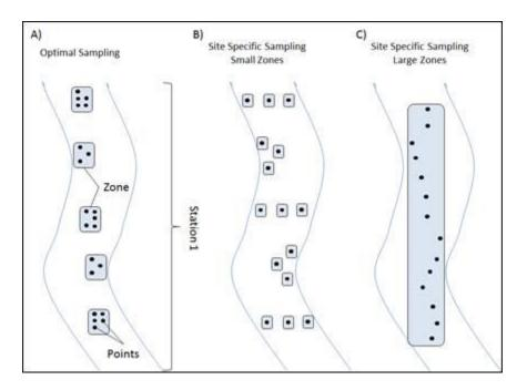
**Figure 8.** Diagram to exemplify determination of sampling zones based on site differences. A) ideal sampling set up based on availability of different depositional zones (~1m<sup>2</sup>); B) in sites with only random small pockets of sediment; and C) in sites where most of the stream bed is characterized by sedimentary or organic substrate.
