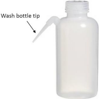
Figure 18. Removing the tip of the 500 mL wash bottle helps makes rinsing easier and increases water pressure. This tip pulls easily out of the main body of the wash bottle.
