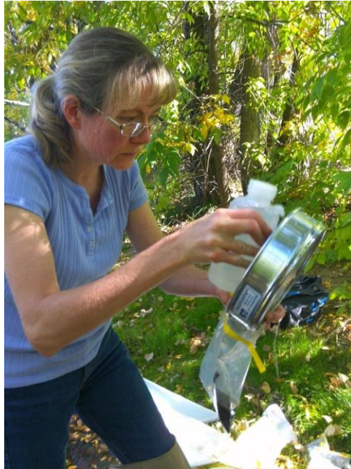
Figure 31. A field technician rinses the sample from the sieve into the open container with the 500 mL wash bottle.
