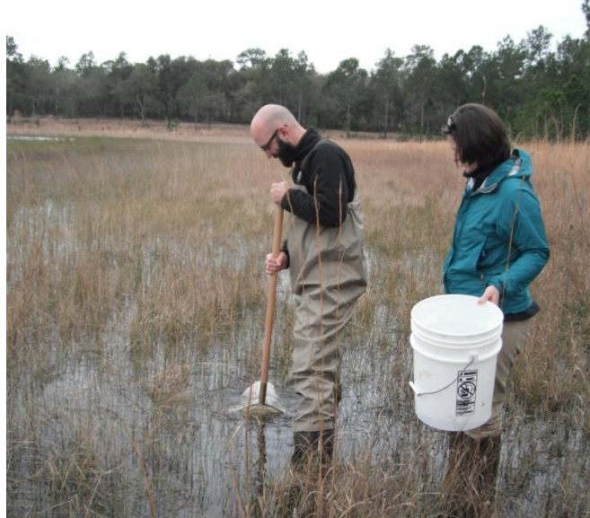
Figure 28. Field technicians demonstrate the sweep technique in a littoral area. The D-frame net must remain submerged and close to the substrate throughout the entire sweep.
