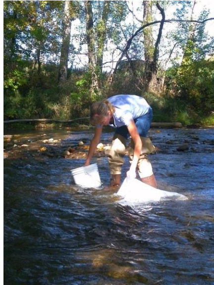
Figure 15. A field technician holds the Surber net on the stream bottom, and keeps the bucket nearby for depositing rocks from the base of the Surber.
