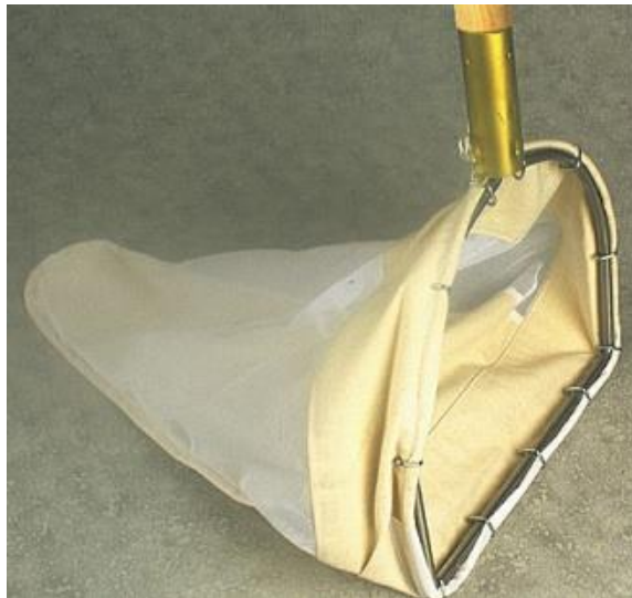
Figure 27. D-frame net, used for sweep samples in vegetation and silty habitats.
