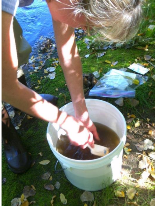
Figure 17. A field technician scrubs rocks from the Surber sample into the 3 gallon bucket
