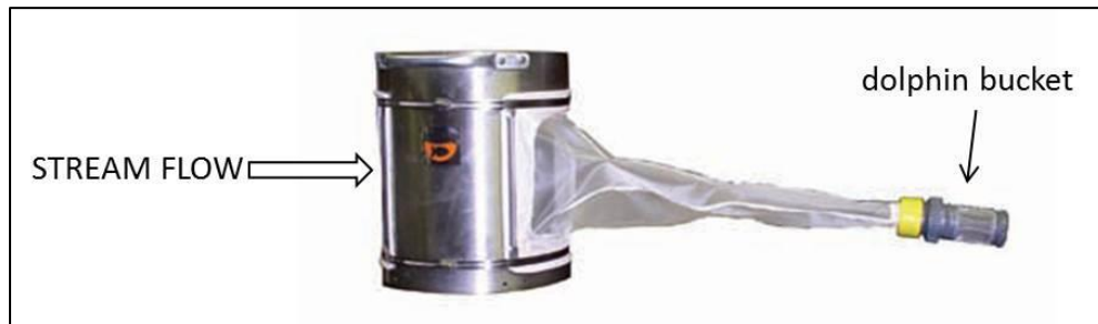
Figure 25. Hess sampler with collection net and dolphin bucket
