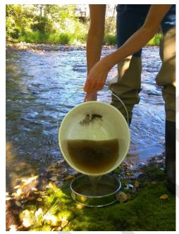
**Figure 25.** A field technician carefully pours water from the 3 gallon bucket into the sieve
