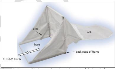
**Figure 12.** Diagram of Surber sampler set-up. The inside of the base is the sample area of the stream bottom  $(0.09 \text{ m}^2)$
