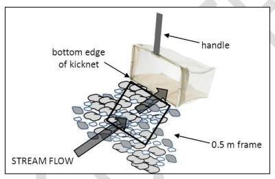
Figure 22. Example of modified kicknet setup
