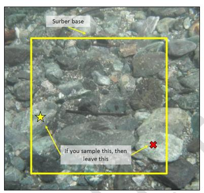
Figure 15. Cobble selection at Surber edges
