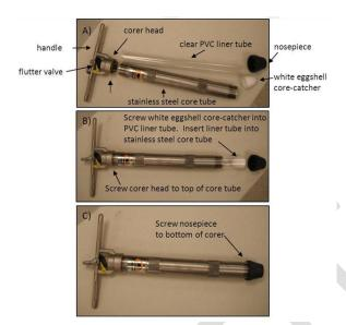
**Figure 20.** Hand-corer assembly: A) Disassembled corer. B) Partially assembled corer. C) Assembled corer. Note: the nosepiece may be stainless steel (not black Lexan as in photo) in some domains
