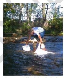
**Figure 14.** A field technician holds the Surber net on the stream bottom, and keeps the bucket nearby for depositing rocks from the base of the Surber
