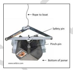
Figure 18. Example of a petite ponar setup
