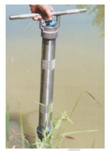
**Figure 21.** Push the hand corer through the water and into the sediments at a 90° angle
