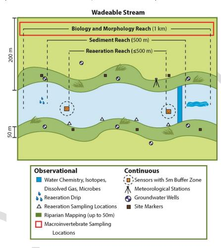
Figure 9. A generic wadeable stream site layout with macroinvertebrate sampling locations.
