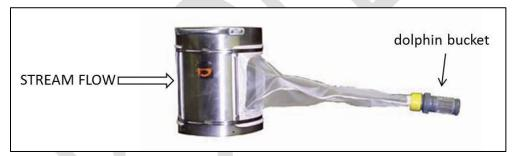
Figure 23. Hess sampler with collection net and dolphin bucket
