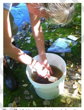
**Figure 17.** A field technician scrubs rocks from the Surber sample into the 3 gallon bucket
