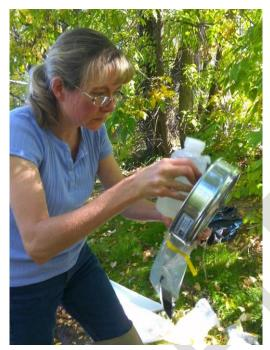
**Figure 26.** A field technician rinses the sample from the sieve into the open container with the 500 mL wash bottle
