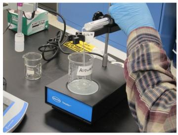
Figure 10. Expelling acid from digital titrator set-up into a temporary acid waste container
