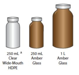
**Figure 2.** Water chemistry bottle types. <sup>a</sup> indicates sample bottles that will remain at NEON Domain Support Facilities to be analyzed. These bottles are labeled with different labels (Figure 4b) and bottles can be re-used. 125 mL bottles may be used if less volume is needed – site specific.
