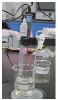
**Figure 11.** Titration setup with digital titrator, stir bar, pH meter, and temperature probe
