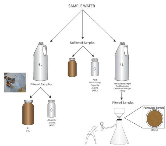
**Figure 3.** Flowchart of Water Chemistry Sample Collection and Filtration.  $\Diamond$  Indicates 250 mL, wide-mouth sample bottles that remain at the Domain Support Facility for analysis. Letters in parenthesis indicate the codes that correspond to the chemistry labels (see Figure 4 a and b).
