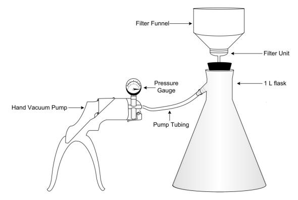
Figure 7. Filter apparatus setup for particulates. Includes the hand vacuum pump, attached to the filter flask and filter funnel/manifold.
