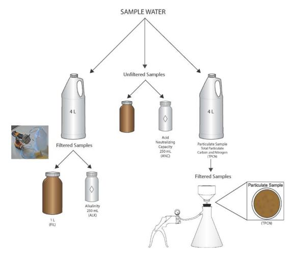
\* Indicates 250 mL, wide-mouth sample bottles that remain at the Domain Support Facility for analysis. Letters in parenthesis indicate the codes that correspond to the chemistry labels (see **Figure 4** a and b).
