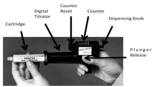
Figure 8. Inserting titrant cartridge into digital titrator. Photo from the Hach digital titrator manual.
