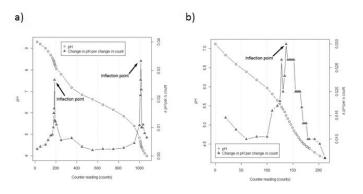
**Figure 12.** Example of inflection point titration using a digital titrator of a) a high alkalinity sample and B) a low alkalinity sample. Note difference in Y-axis scale. (Modified from USGS TWRI Book 9, Alkalinity, Version 3.0 7/2006).
