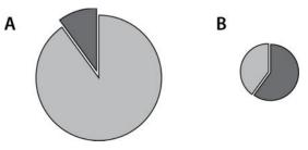
**Figure 5.** Creating wedge-shaped subsamples from cross-sectional disks from relatively large disks (A), and relatively small disks (B). In both A and B, the dark grey area is approx. 100 g, and the light grey is discarded.
