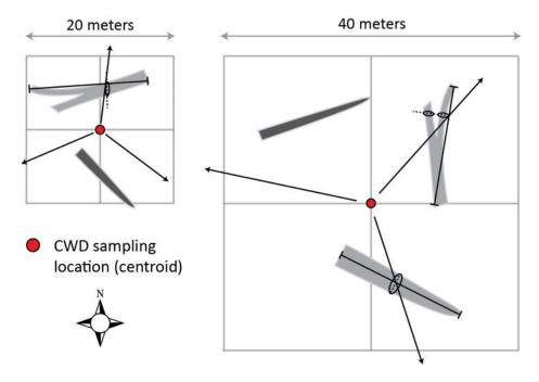
**Figure 1.** Illustration of three randomly oriented LIDS transects (arrow vectors) superimposed over a 20m x 20m plot (*left*), and a 40m x 40m plot (*right*). There is a 3m gap between the sampling location (i.e. the plot centroid), and the start of each transect
