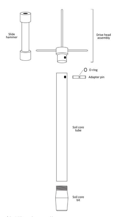
Figure 7. Component parts of the Giddings soil core assembly.
