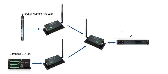
To avoid data collisions in the LC base station, the modems need to be configured as follow:
