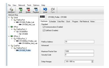
m) Right-click CR1000\_Profiler to add a second CR1000 as a slave device. Rename it as CR1000\_MetStation with PakBus Address 20
