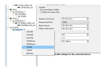
With CR1000 selected, click Rename in the main toolbar and change the name to CR1000\_Profiler and in the Hardware tab, change the "PakBus Address" to 10
