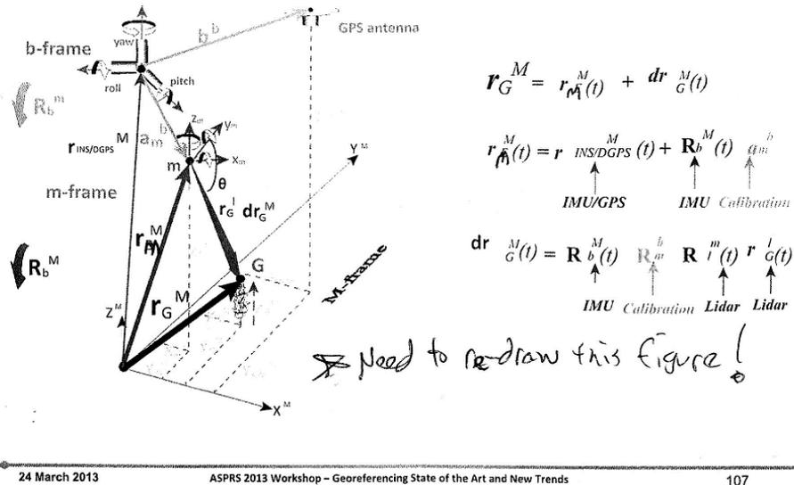
Figure 14. Computation of Ground Coordinates with Direct Georeferencing.
