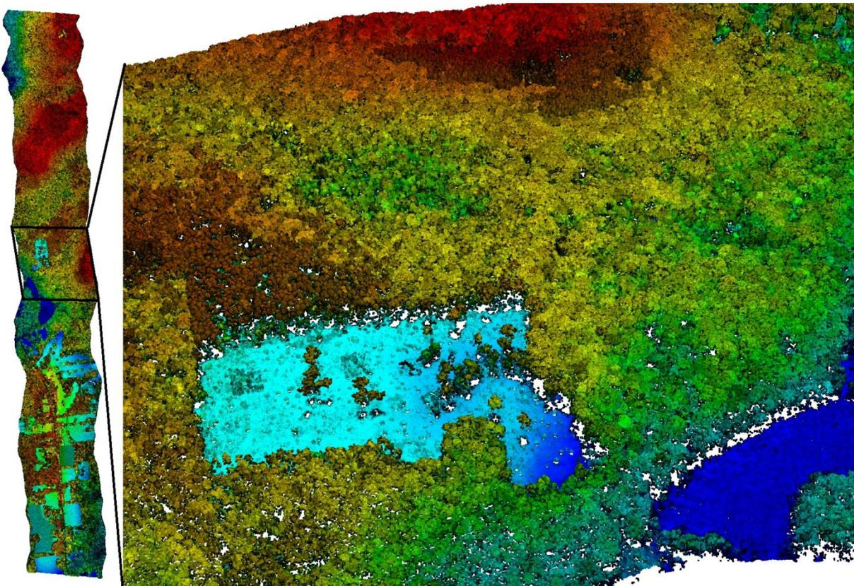
**Figure 3.** Example Discrete Return LiDAR Level 1 Point Cloud Product colored by absolute elevation. The left side of the figure shows the entire flight line and the right side shows a close up view of the forest as viewed in 3D from an oblique side angle.
