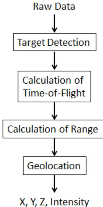
**Figure 11.** High-level discrete LiDAR processing flow.
