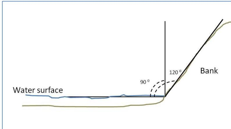
**Figure 46** How Bank Angle is Measured
