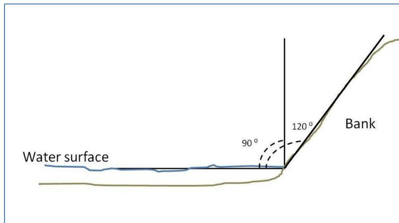
**Figure 42. How Bank Angle is Measured**
