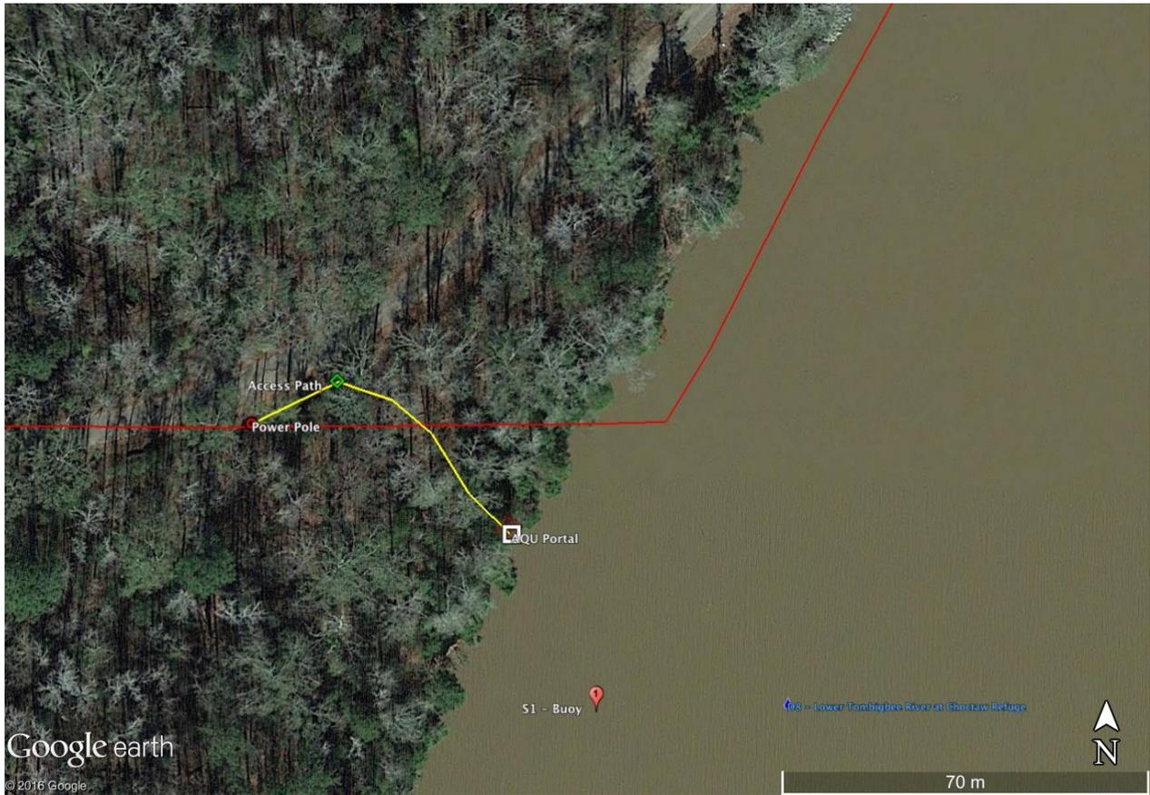
**Figure 53. Map showing access path (starting at green diamond) and continuing with conduit run (yellow) to portal location.**
