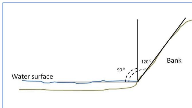
Figure 9. How Bank Angle is Measured
