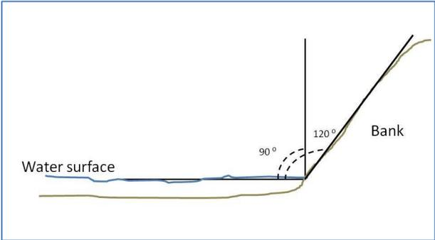
**Figure 64** How Bank Angle is Measured
