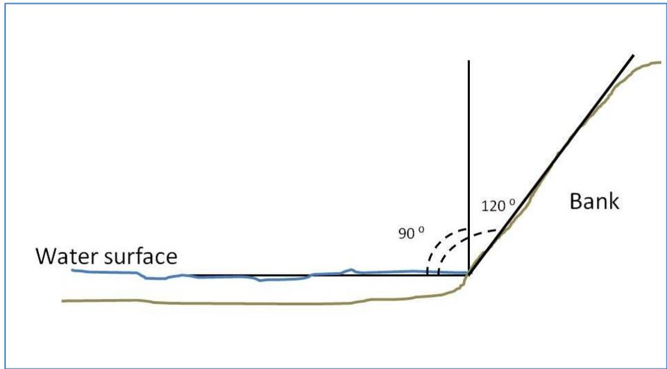
**Figure 22** How Bank Angle is Measured
