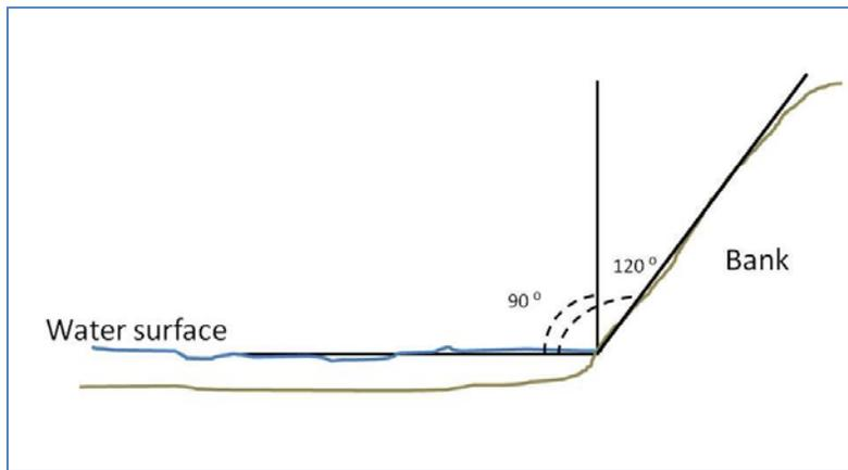
**Figure 9** How Bank Angle is Measured
