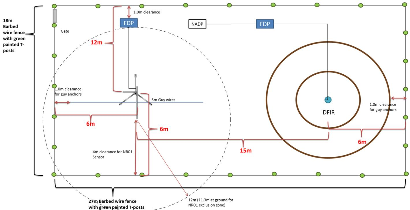
**Figure 6.** Schematic of met station, wet deposition collector and DFIR that includes cattle fence location relative to sensors and infrastructure.
