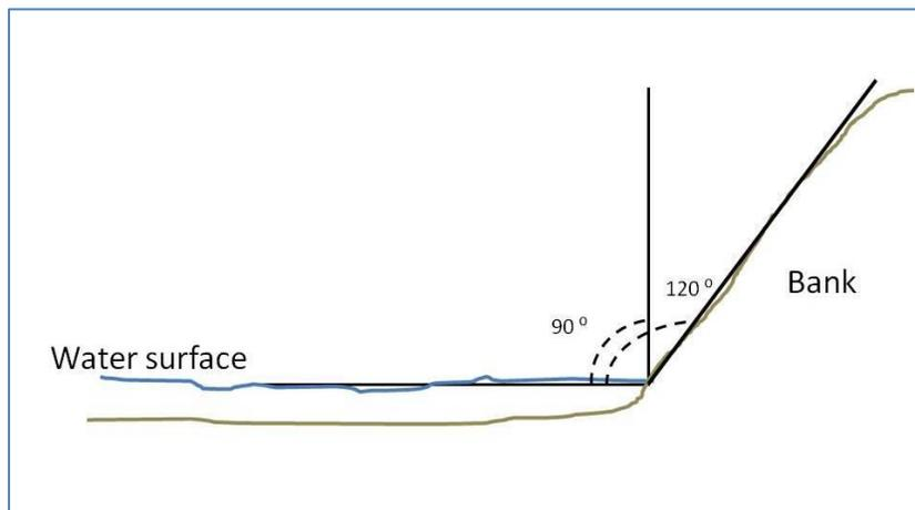
**Figure 9** How Bank Angle is Measured
