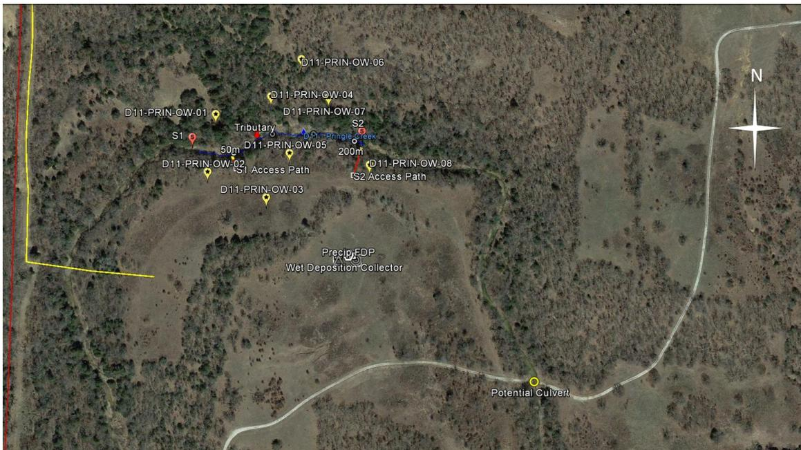
Figure 19 Site map showing proposed culvert installation (yellow circle) where road passes through the creek.
