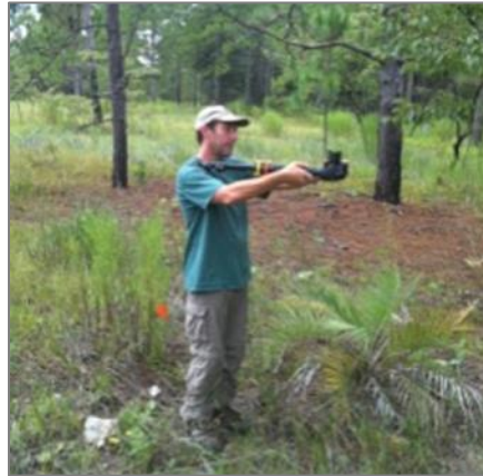
Figure 7. A field researcher acquiring an upward-facing DHP with the monopod/camera ensemble held at shoulder height
