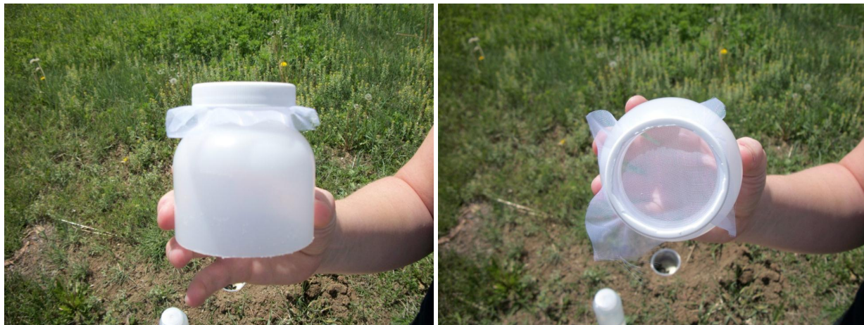
Figure 8. 300 \mu m mesh filter fitted to the top of a Nalgene bottle
