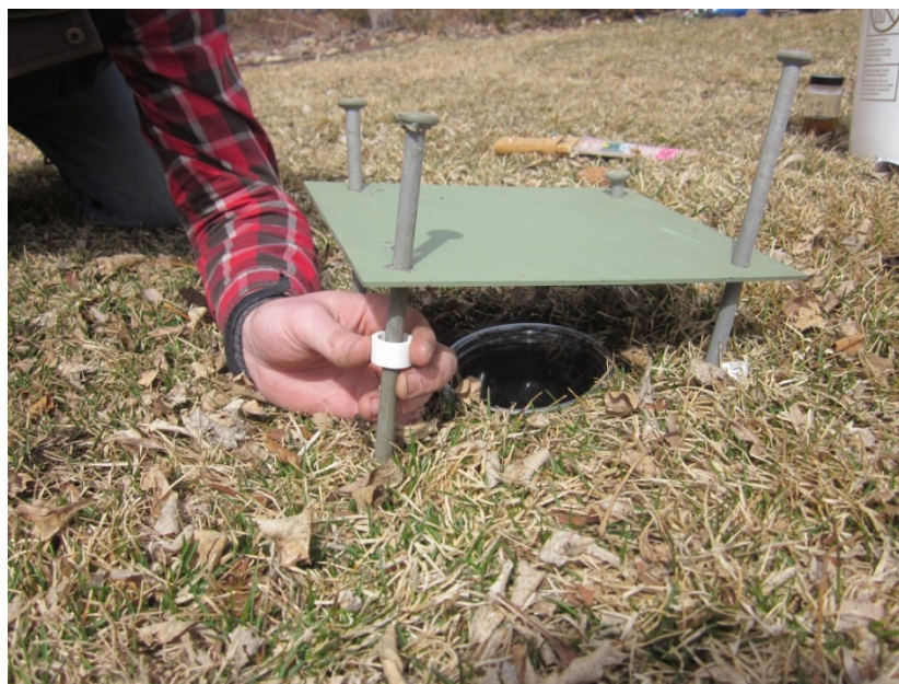
Figure 6. Installing pitfall lid with spacers. Note that the container is flush with the ground. If washers are used, they should be placed between the ground and the bottom of the spacer.
