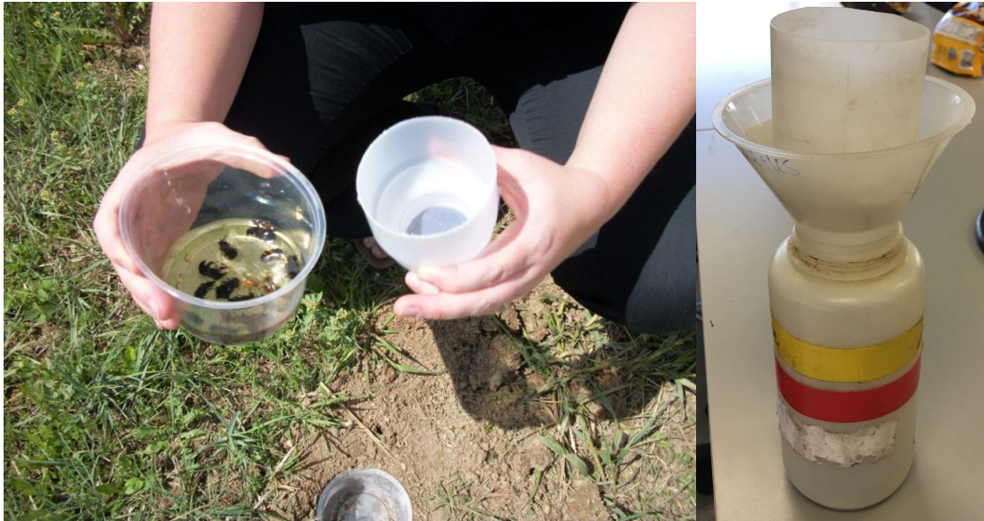
Figure 9. Preparing to filter out specimens from collecting fluid (pictured left). Optionally, a funnel can be placed between the filter assembly and the Nalgene waste container (pictured right).
