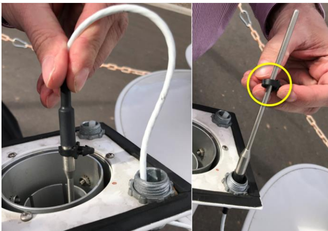
Figure 15. Remove PRT from Assembly
