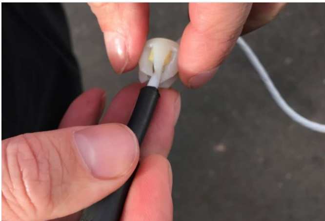
Figure 18. Remove Cable Clamp from PRT Cable
