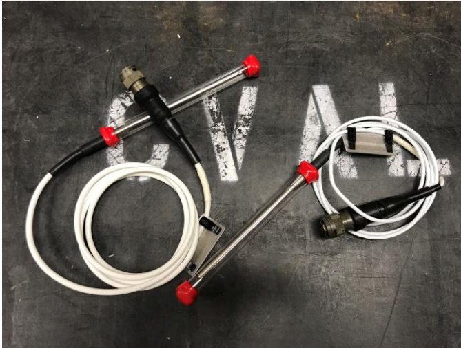
Figure 19. Cap PRT Probe for Shipping/Handling
