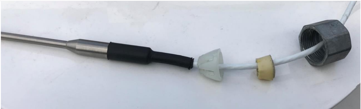
Figure 20. Reverse Order to Reassemble PRTs with AATs
