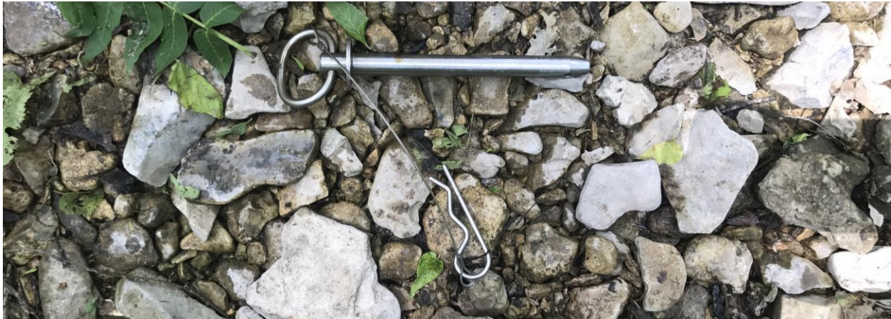
Figure 11. Multisonde/PRT PVC Housing Cap Clip (Removed from PVC Housing Cap) (D06, KINGS)
