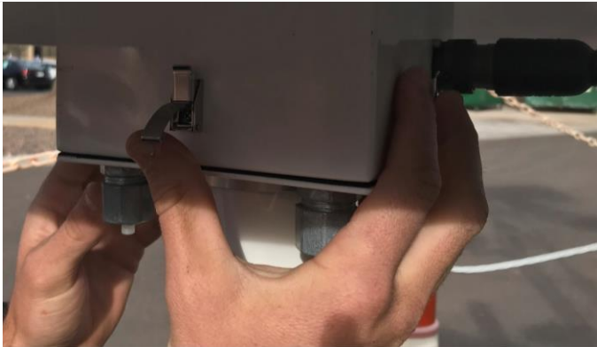
Figure 12. Unlatch the Four Locking Latches
