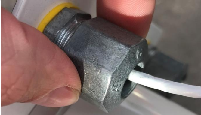
Figure 13. Unthread the Strand Relief Gland with the PRT Cable
