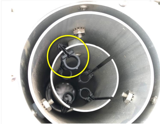
Figure 16. Decontaminate the AAT Assembly & Return Black PRT Retaining Clip
