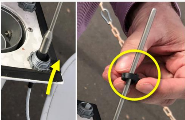
Figure 21. Reassemble PRT and Install Black PRT Retaining Clip
