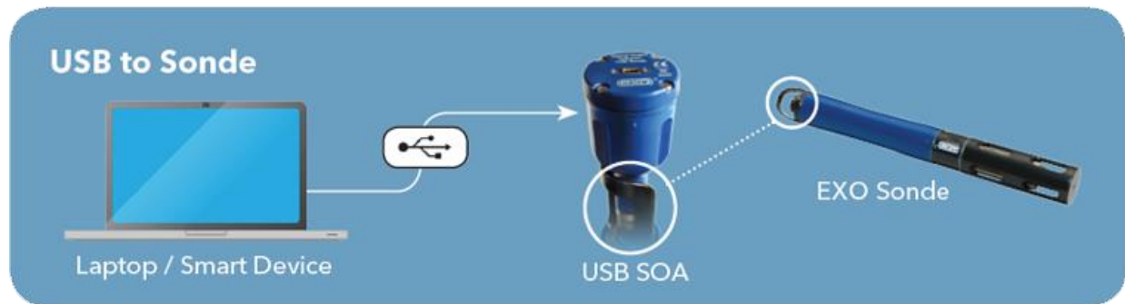
Figure 1. USB to Sonde Connection Method
