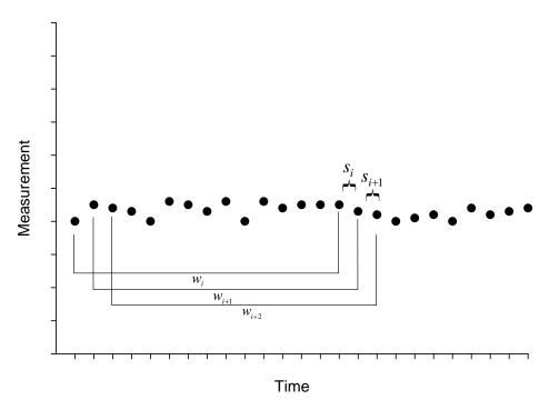
Figure 1: How windows step though a time series of observations. Here the window, w, is defined as 15 observations and the step size, s, is 1.
