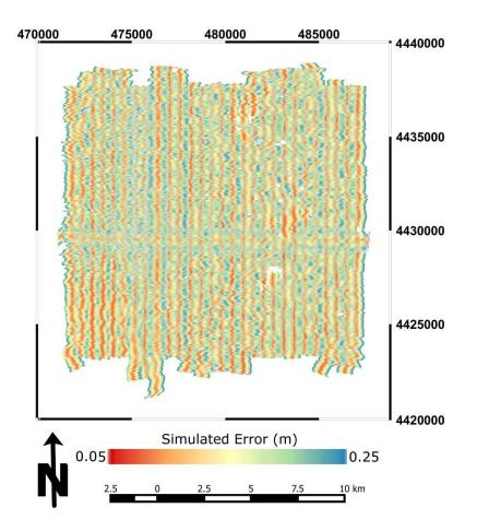
**Figure 167**. Simulated error from lidar sensor hardware sources for the October 8th 2013 survey of the city of Boulder, Colorado.
