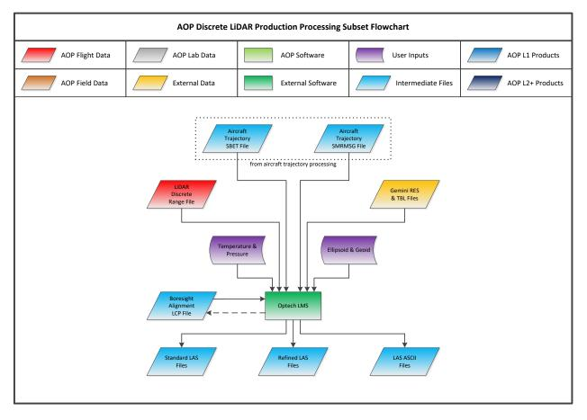
Figure 15. High-Level Discrete Return LiDAR Processing Flowchart.
