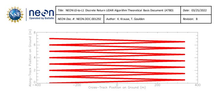
Figure 9. LiDAR Scan Pattern on the Ground for a Nominal Collection.
