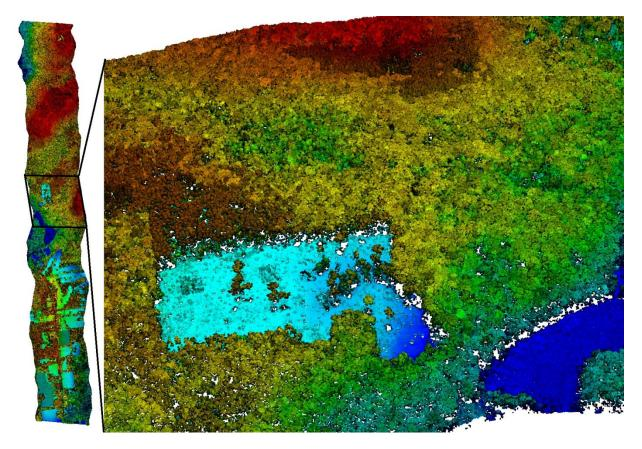
Figure 3. Example Discrete Return LiDAR Level 1 Point Cloud Product colored by absolute elevation. The left side of the figure shows the entire flight line and the right side shows a close up view of the forest as viewed in 3D from an oblique side angle.
