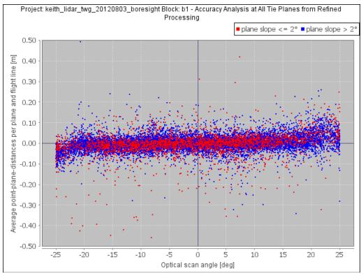
Figure 24. Difference in tie planes versusscan angle after boresight alignment calibration.
