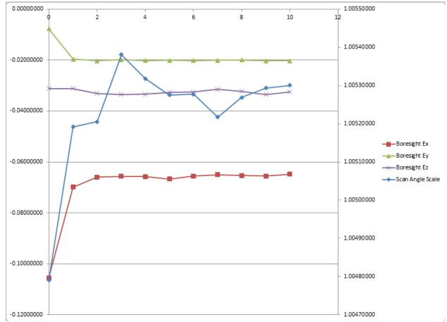
**Figure 26**. Bore sight alignment calibration LCP values for a series of 10 consecutive self-calibrations with parameter updates for each iteration.
