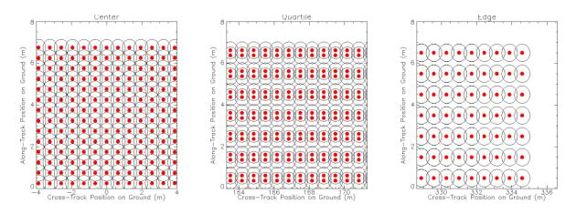
Figure 10. LiDARPoint Spacing on the Ground for a Nominal Collection.
