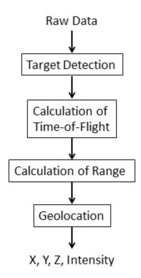
Figure 11. High-level discrete LiDAR processing flow.
