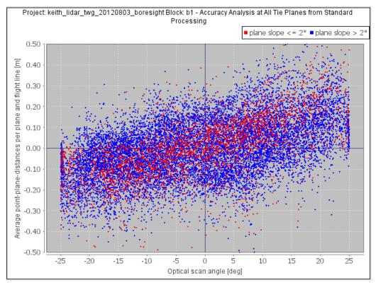
Figure 23. Difference in tie planes versus scan angle before boresight alignment calibration.
