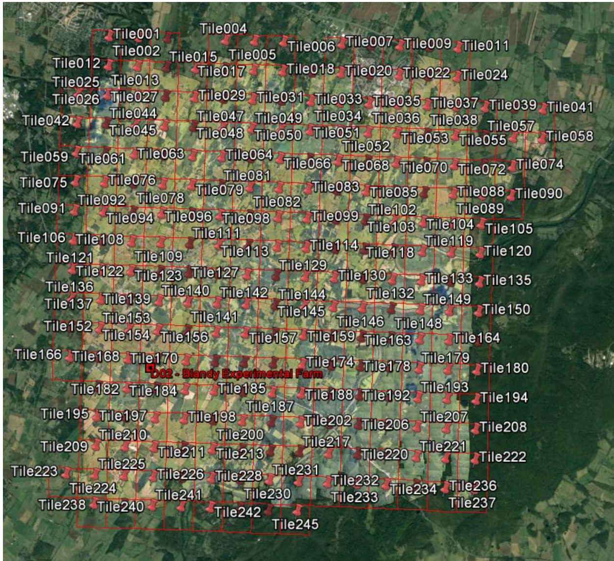
Figure 5. A low-resolution mosaic of the site BLAN showing the boundaries of the tiles (in red). The image is displayed in Google Earth that provides the background. The pushpins identify the individual tiles.
