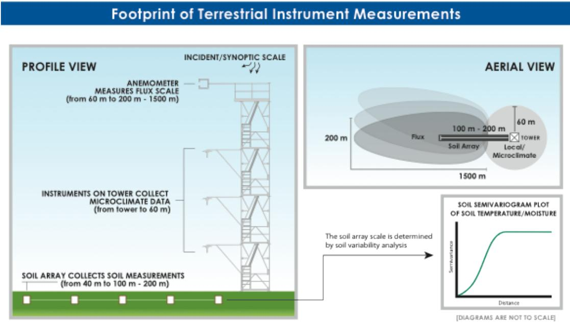
**Figure 17: Design for terrestrial instrument measurements including profile view of instrumented tower and soil array, aerial view of the measurement area, and a schematic soil semivariogram plot, used to determine the spacing between soil samples.**
