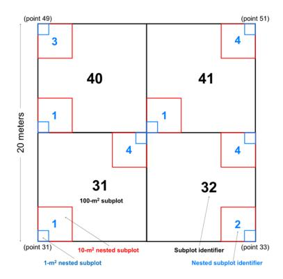
**Figure 2**. A schematic of the multi-scale plot for sampling plant species diversity and abundance (Peet et al. 1998). The plot is nested within a larger plot designed to accommodate other NEON protocols such as soils, beetles, and plant biomass and productivity; the corner points and associated subplot identifiers are numbered to correspond to this larger plot.
