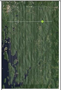
Figure 4.1.2. Flight lines over Harvard Forest at nominal 1000m AGL
