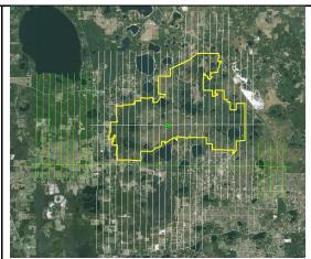
Figure 4.5.2. Priority 1 flight lines (white) and priority 2 flight lines (green) over Ordway-Swisher Biological Station at nominal 1000m AGL.
