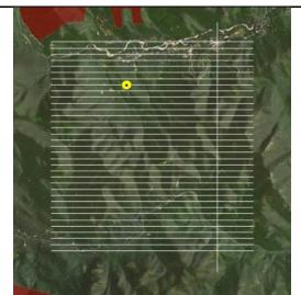
Figure 4.2.2. Flight lines over Bartlett Experimental Forest at nominal 1000m AGL
