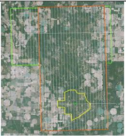
Figure 4.7.2. Flight lines over Jones Ecological Research Center at nominal 1000m AGL.
