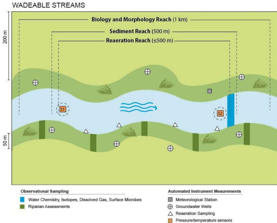
**Figure 4.** Generic diagram for an AQU site showing sampling locations in a wadeable stream system. Note: the sensor locations are not typically installed as depicted; sediment stations 1 and 2 are divided by the biological reach center not the midpoint between sensors.
