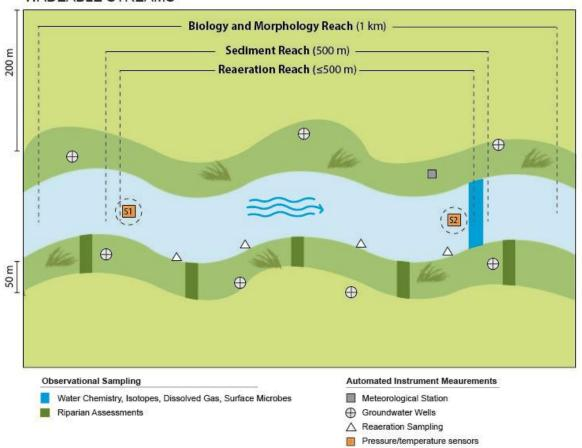
**Figure 4.** Generic diagram for an AQU site showing sampling locations in a wadeable stream system. Note: the sensor locations are not typically installed as depicted; sediment stations 1 and 2 are divided by the biological reach center not the midpoint between sensors.
