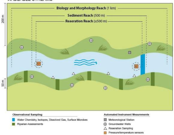
**Figure 6.** Generic diagram for an AQU site showing sampling locations in a wadeable stream system. Note: the sensor locations are not typically installed as depicted; sediment stations 1 and 2 are divided by the biological reach center not the midpoint between sensors.
