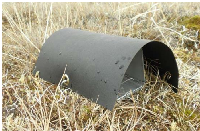
Figure 16. Folding Sherman trap (3"x3.5"x9") covered with 12"x12" tar paper cover in Barrow, AK - from Ott 2012. Credit: Kaithryn Ott.
