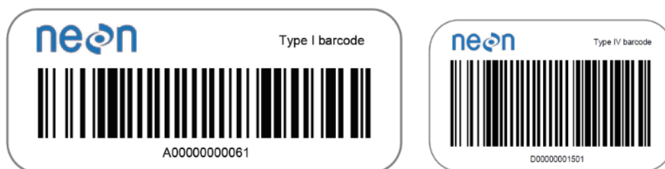
Figure 9. An example of a Type I and a Type IV barcode. Type I barcodes should be used on coin envelopes for hair and whisker samples, and are large-size and field-tolerant with a prefix of 'A' followed by 11 numbers. Type IV barcodes should be used on all 2mL vials and placed on the back of voucher labels. Type IV barcodes are -80 tolerant and have a prefix D followed by 11 numbers.
