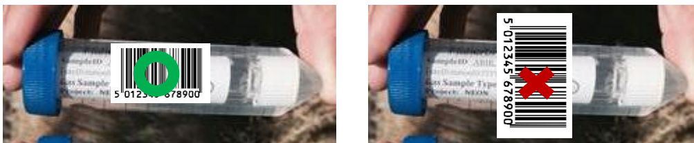
Figure 8. Diagram showing appropriate orientation of barcodes on vials to allow for scanning.
