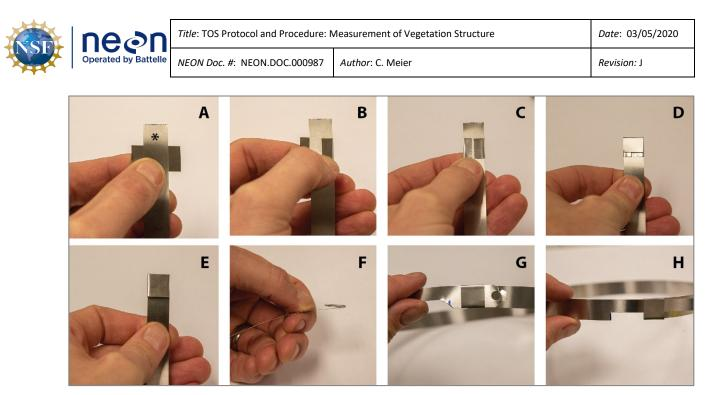
**Figure 23**. Fabricating the dendrometer band buckle with the collar after fitting the band to the tree and cutting to the desired length. The asterisk in **A** denotes the outward-facing side of the band marked in the previous step.
