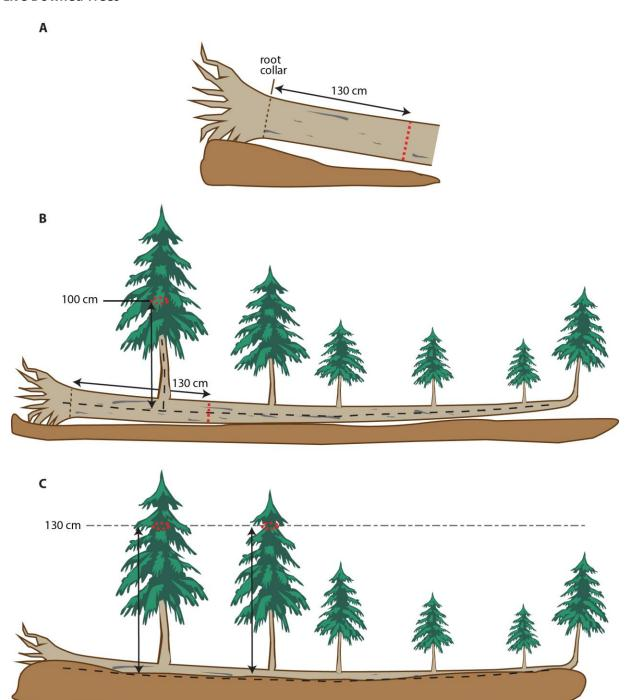
Figure 13. Stem diameter measurement guidelines for live, downed trees.
