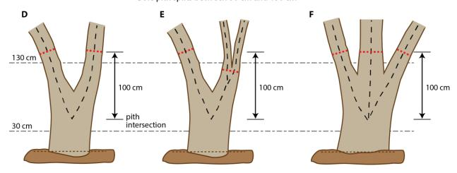
Figure 12. Stem diameter measurement guidelines for multi-bole trees with pith splits.
