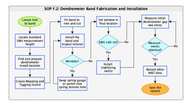
**Figure 21**. SOP F.2 workflow diagram for dendrometer band installation in the field, and initial measurements. Diagram supports and does not replace protocol text; most common workflow is outlined.
