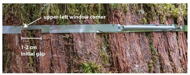
**Figure 24**. Installed dendrometer band with a 1-2 centimeter initial gap in the measurement window. The band is rotated such that the entirety of the measurement window and the spring are fully appressed to a smoothed section of the bole.
