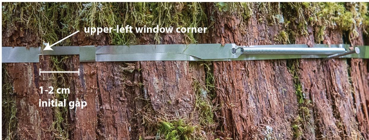
**Figure 25.** Installed dendrometer band with a 1-2 centimeter initial gap in the measurement window. The band is rotated such that the entirety of the measurement window and the spring are fully appressed to a smoothed section of the bole.
