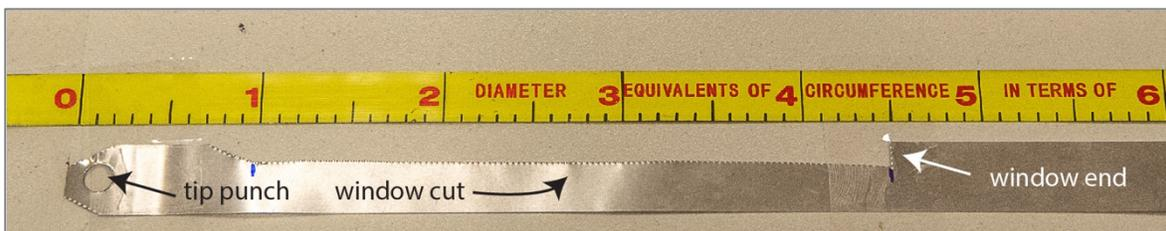
**Figure 5.** Completed preparation of a dendrometer band showing tip punch (left), window cut (center), and window end from which measurements are made in the field (right). Note the DBH tape is taped to the work surface with diameter centimeter equivalents (dcm) facing up, not centimeters.
