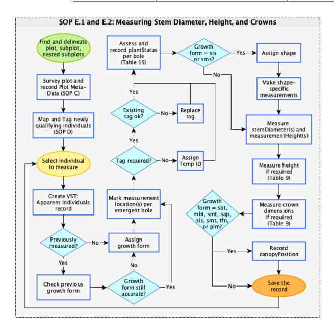
**Figure 10**. SOP E.1 and E.2 workflow diagram for stem diameter, height, and crown dimension measurements collected from apparent individuals. Diagram supports and does not replace protocol text; most common workflow is outlined.
