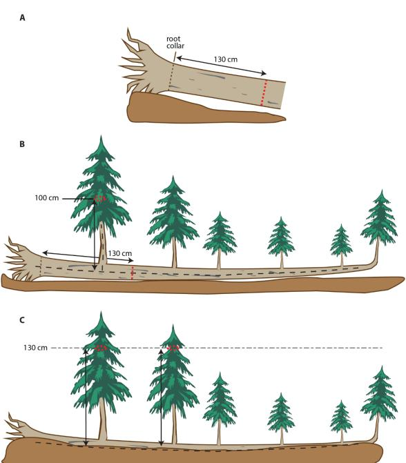
Figure 13. Stem diameter measurement guidelines for live, downed trees.
