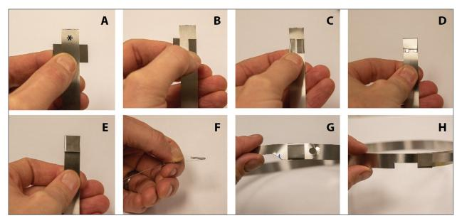
**Figure 24**. Fabricating the dendrometer band buckle with the collar after fitting the band to the tree and cutting to the desired length. The asterisk in **A** denotes the outward-facing side of the band marked in the previous step.
