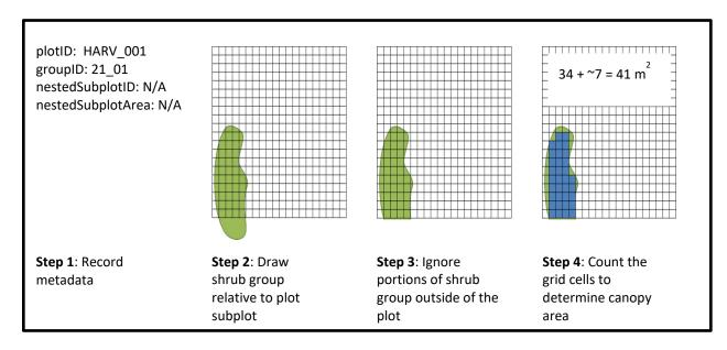
Figure 20. Example of graph paper method for estimating shrub group area within a 20 m x 20 m subplot. In this example, canopyArea =  $41 \text{ m}^2$ .
