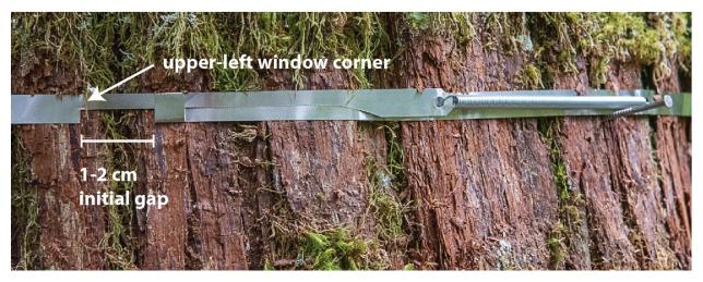
**Figure 25**. Installed dendrometer band with a 1-2 centimeter initial gap in the measurement window. The band is rotated such that the entirety of the measurement window and the spring are fully appressed to a smoothed section of the bole.
