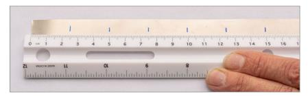
**Figure 3**. Dendrometer band material marked every 2.5 cm for cutting 'collars' in preparation for installation in the field.
