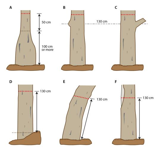
Figure 11. Stem diameter measurement guidelines for irregular single-bole trees. The lowest dashed line represents ground level from which the desired measurement height is referenced. The thick dashed red line shows the desired measurement height above ground level. Tags are typically placed 10 cm above the measurement height.
