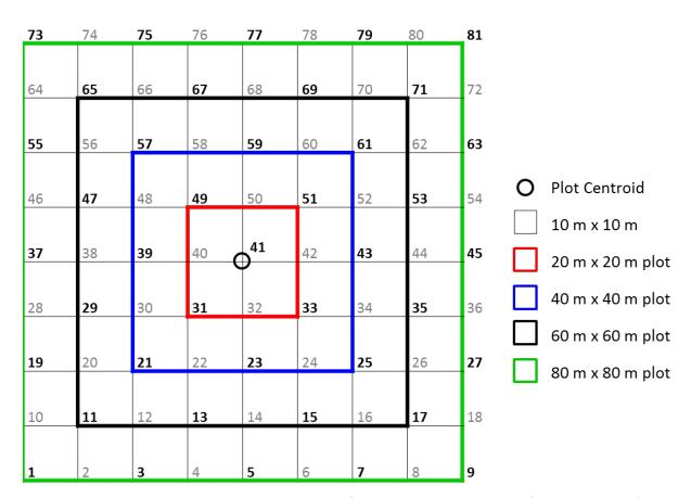
**Figure 27**. Plot map, illustrating how NEON base plots of various sizes are constructed from 10 m x 10 m 'modules.' The SW corner of each 'module' receives a pointID number; bold numbers indicate pointIDs that may receive physical markers.
