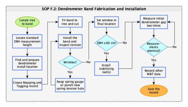
**Figure 22**. SOP F.2 workflow diagram for dendrometer band installation in the field, and initial measurements. Diagram supports and does not replace protocol text; most common workflow is outlined.
