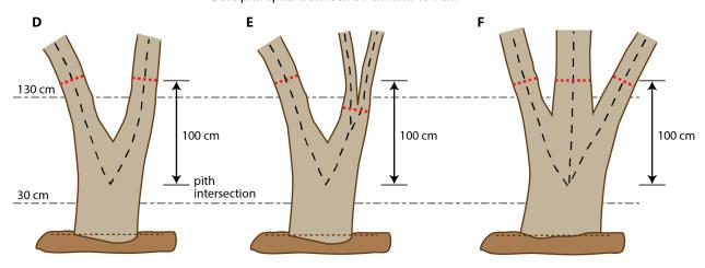
**Figure 12**. Stem diameter measurement guidelines for multi-bole trees with pith splits. See **Figure 15** for Shrub guidance.
