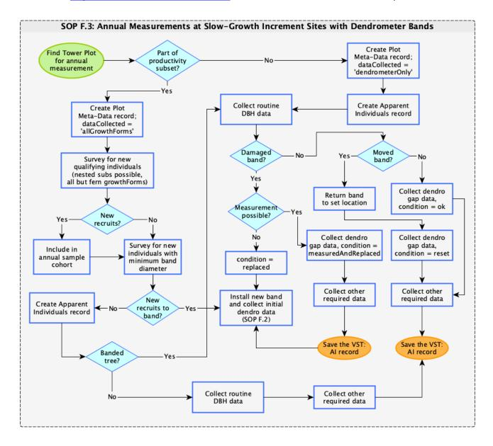
**Figure 26**. SOP F.3 workflow diagram for annual measurements in Tower Plots at slow-growth increment sites with dendrometer bands. Diagram supports and does not replace protocol text; most common workflow is outlined.
