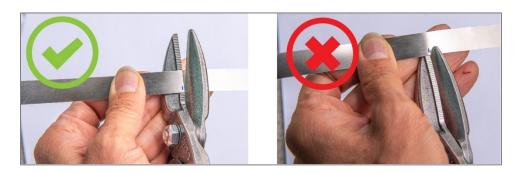
**Figure 4**. (*Left*) Correct metal-snip technique for cutting the measurement window in a dendrometer band. (*Right*) Incorrect technique using the tip of the metal snips will result in burrs and band deformation.
