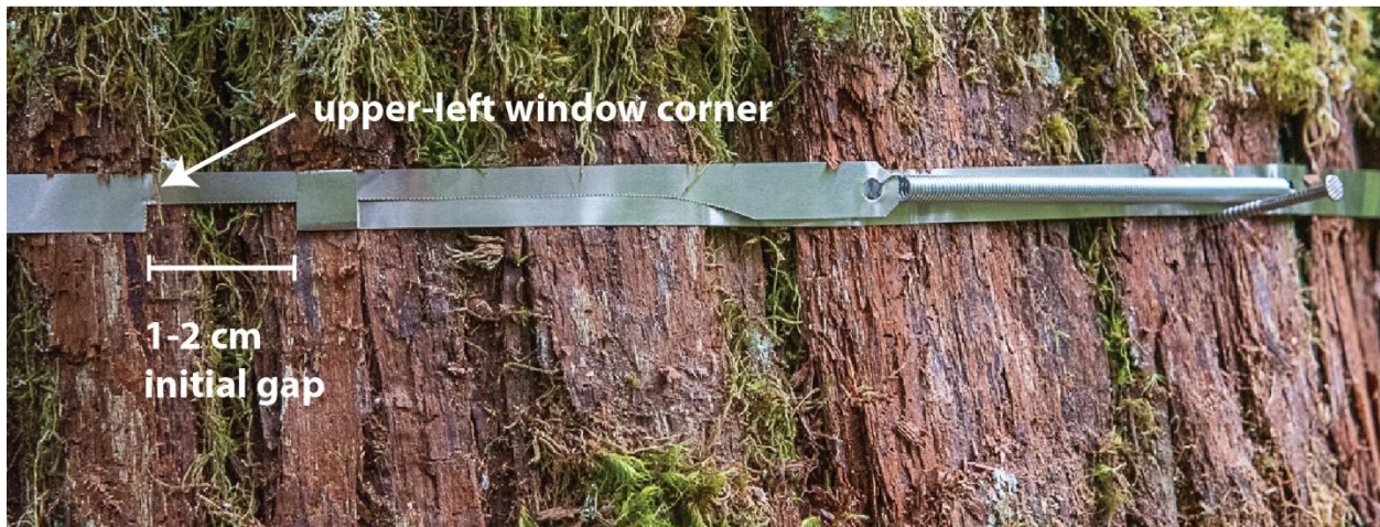
Figure 29. Installed dendrometer band with a 1–2 centimeter initial gap in the measurement window. The band is rotated such that the entirety of the measurement window and the spring are fully appressed to a smoothed section of the bole.
