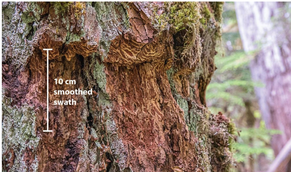
Figure 27. Preparation of the bole surface for dendrometer band installation on a deeply fissured Douglas Fir ( Pseudotsuga menziesii ) at the D16 WREF site.
