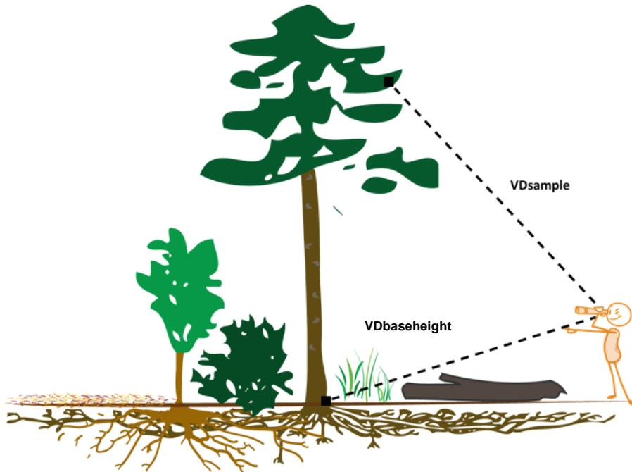
**Figure 12.** Measuring sample height using a laser rangefinder.
