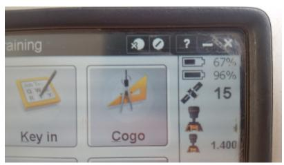
Figure 40. Battery status display
