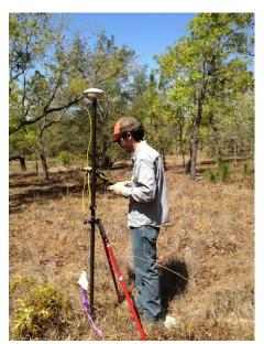
**Figure 14.** GeoXH 6000 set up for high accuracy data collection.
