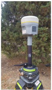
Figure 37. Base station setup.
