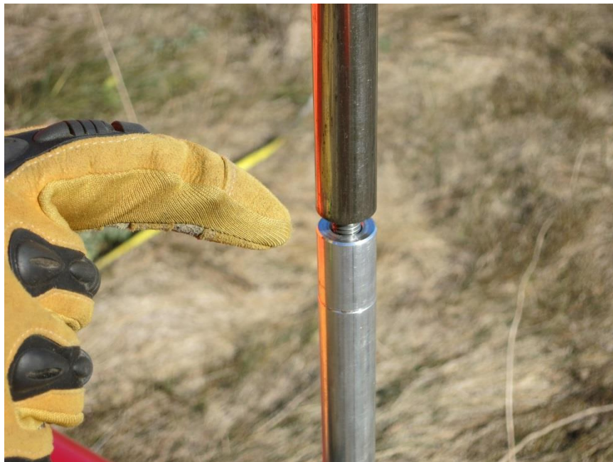
Figure 14. Picture of rod assembly sections separating while driving the monument, be sure to tighten before continuing.
