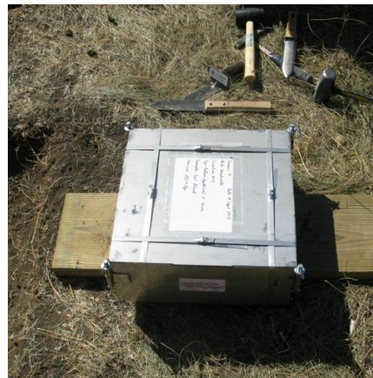
Figure 4. Intact block of soil during (left panel) and after (right panel) collection at D09 Woodworth.
