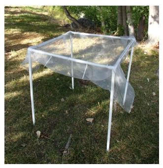
Figure 9. Fully constructed elevated litter trap.
