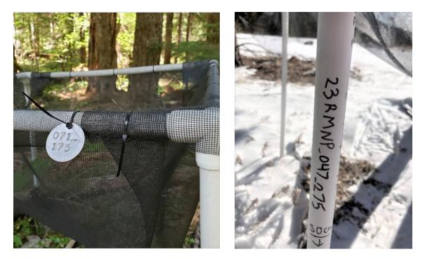
Figure 10. Label elevated traps with the trapID either written on a leg with permanent marker (right) or stamped into a metal tree tag (left)
