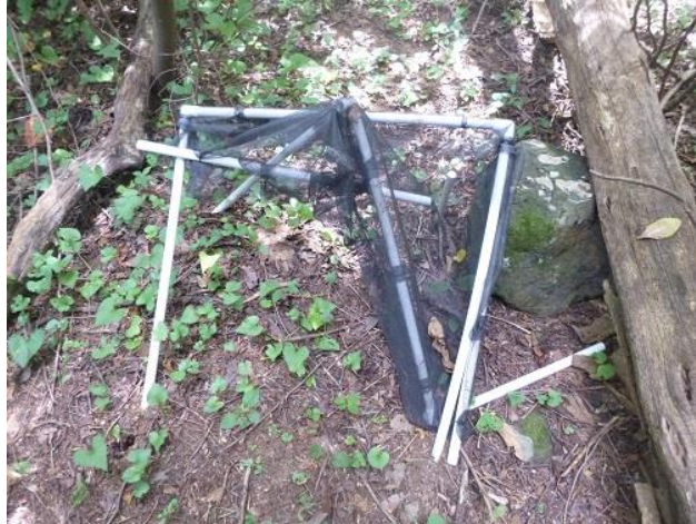
Figure 28. PVC elevated trap destroyed by bears at SCBI.
