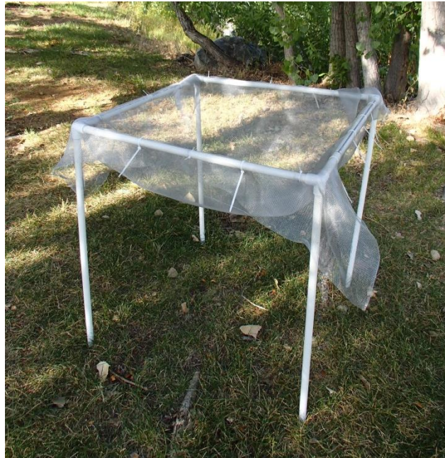
Figure 9. Fully constructed elevated litter trap.
