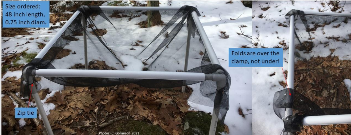
Figure 11. Snap Clamp installation.
