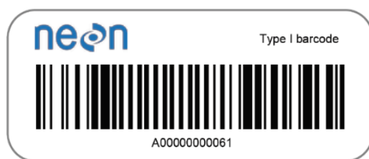
Figure 5. An example of a Type I barcode. These large-size, field-tolerant barcodes have a prefix of 'A' followed by 11 numbers.
