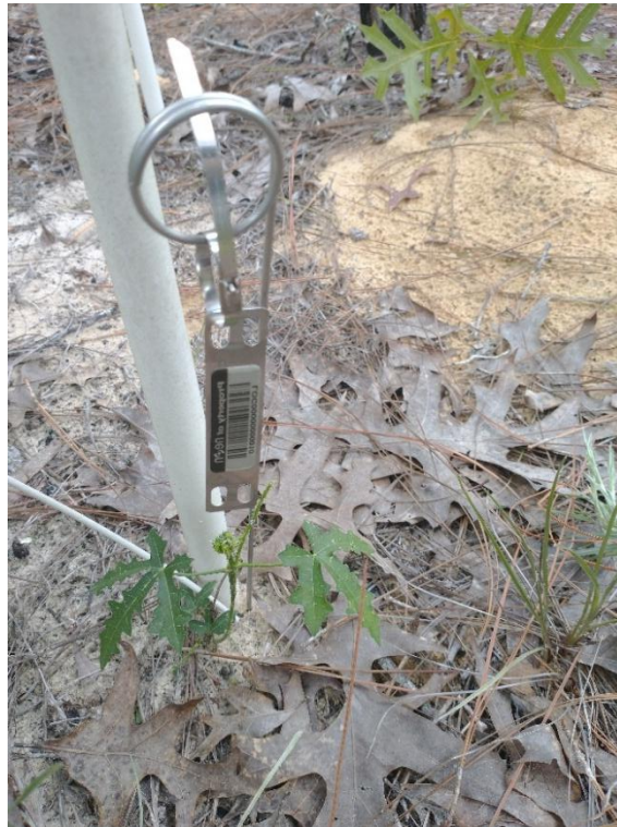
Figure 15. Example of barcode deployed in the field using a pigtail stake.
