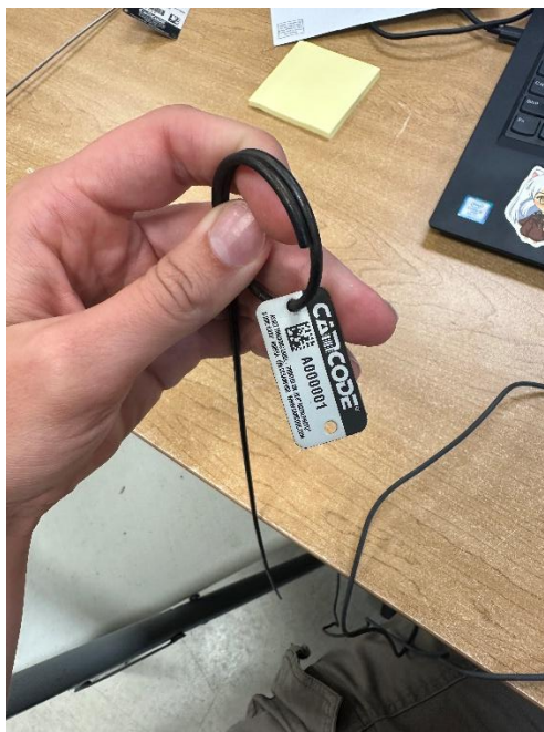
Figure 3. Example field barcode attached to pigtail stake.
