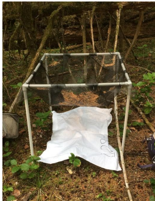
Figure 17. Use of ground cloth to catch trap throughfall.
