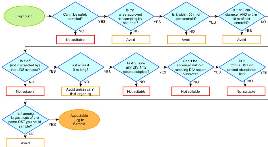
Figure 14. Workflow for determining if a log is appropriate to use for CDW bulk density sampling.
