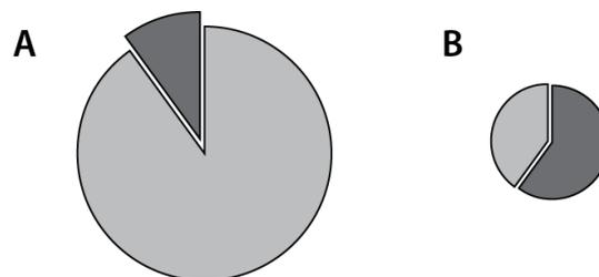
**Figure 17.** Creating wedge-shaped subsamples from cross-sectional disks from relatively large disks (A), and relatively small disks (B). In both A and B, the dark grey area is between 100-400 g, and the light grey is discarded.
