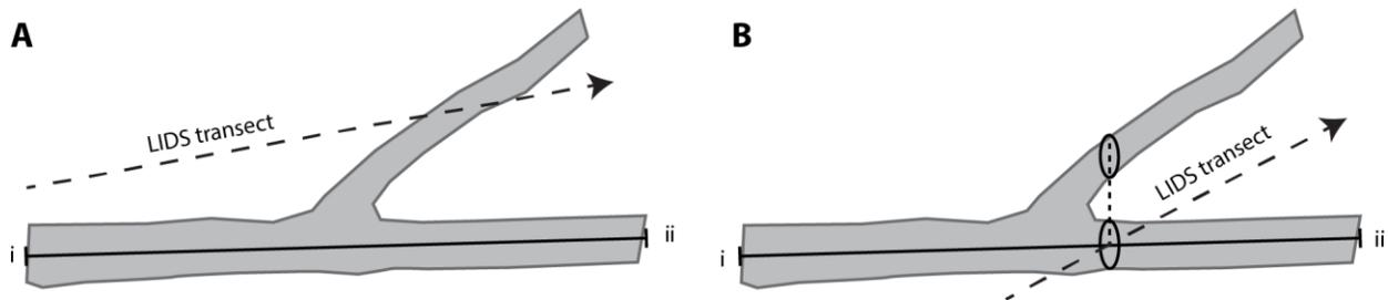
**Figure 12.** A log with a simple fork may be skipped (A) or tallied (B) depending on where the LIDStransect intersects the central axis. (A) The transect misses the central axis, defined as the line between i and ii, and the log is not tallied. (B) The transect intersects the central axis and diameter measurements for the log and fork are made perpendicular to the central axis; the  $RD_E$  of the log + fork are used to determine whether the log is tallied.
