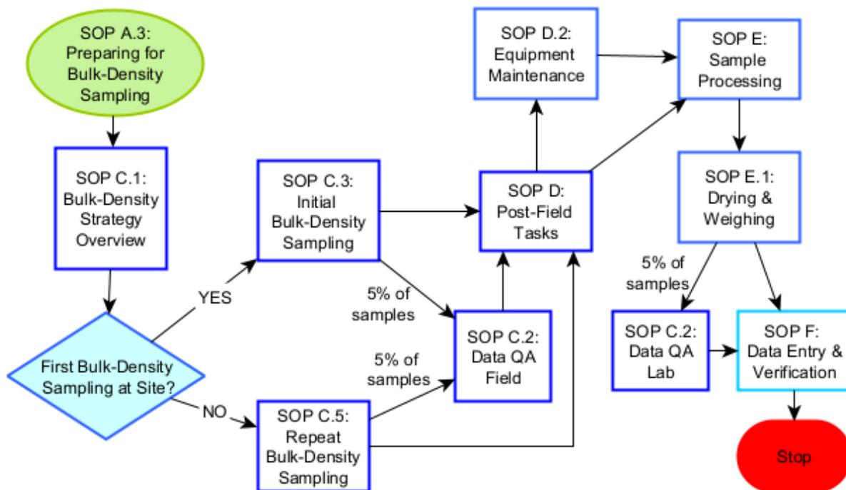
**Figure 3.** High level workflow diagram of Bulk-Density sampling.
