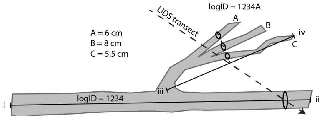
**Figure 13.** LIDS transect intersecting a log with compound forks in two different size categories. Forks in different size categories are assigned unique and related logIDs. The central axis for the main log is defined by the capped line connecting i-ii, and the central axis for the smaller size category compound forked branch is defined by the iii-iv capped line. Measurement locations for each are marked with ellipses.
