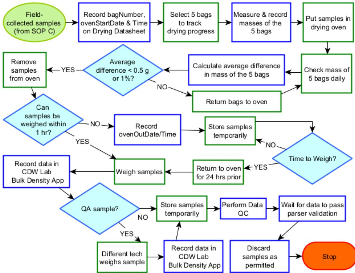
Figure 20. Workflow of CDW Bulk-Density lab process.
