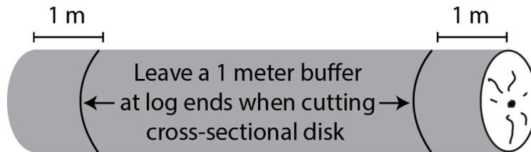
**Figure 15.** A minimum 1 m buffer should be left on either end of a  $\geq 10$  cm diameter CDW piece when cutting a cross-sectional disk for bulk-density sampling. The log depicted is  $> 5$  m length and is sampled from both ends at each of the two sampling timepoints. Qualifying logs  $< 5$  m length are only sampled at one end.
