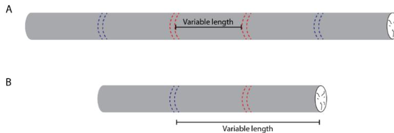
**Figure 18.** Strategy for generating cross-sectional disks from logs re-sampled for bulk density in Bout 2. (A) Logs ≥ 5 m length in Bout 1 and ≥ 3 m length in Bout 2; (B) Logs < 5 m length in Bout 1 and < 3 m length in Bout 2. Pairs of blue dashed lines represent Bout 1 disks, and pairs of red dashed lines indicate Bout 2 disks.
