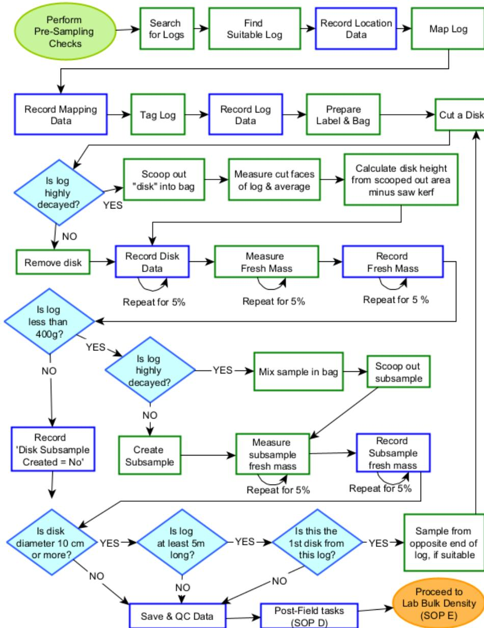
Figure 19. Workflow of CDW Bulk-Density field sampling.
