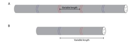
**Figure 18**. Strategy for generating cross-sectional disks from logs re-sampled for bulk density in Bout 2. (A) Logs  $\geq$  5 m length in Bout 1 and  $\geq$  3 m length in Bout 2; (B) Logs < 5 m length in Bout 1 and < 3 m length in Bout 2. Pairs of blue dashed lines represent Bout 1 disks, and pairs of red dashed lines indicate Bout 2 disks.
