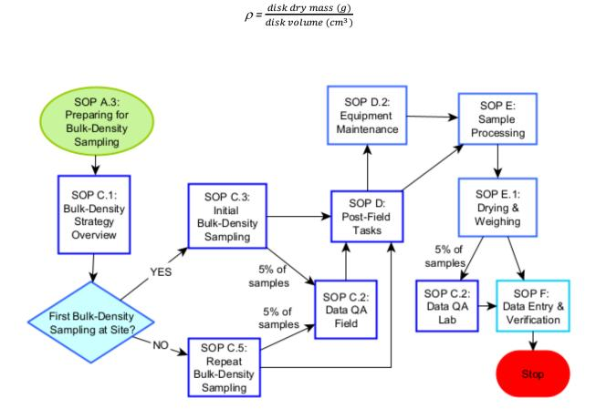
Figure 3. High level workflow diagram of Bulk-Density sampling.
