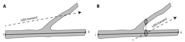
**Figure 12**. A log with a simple fork may be skipped (A) or tallied (B) depending on where the LIDS transect intersects the central axis. (A) The transect misses the central axis, defined as the line between i and ii, and the log is not tallied. (B) The transect intersects the central axis and diameter measurements for the log and fork are made perpendicular to the central axis; the RD<sub>E</sub> of the log + fork are used to determine whether the log is tallied.
