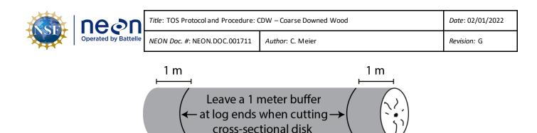
**Figure 15**. A minimum 1 m buffer should be left on either end of  $a \ge 10$  cm diameter CDW piece when cutting a cross-sectional disk for bulk-density sampling. The log depicted is > 5m length and is sampled from both ends at each of the two sampling timepoints. Qualifying logs < 5m length are only sampled at one end.
