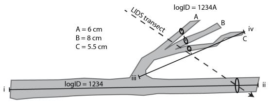
**Figure 13**. LIDS transect intersecting a log with compound forks in two different size categories. Forks in different size categories are assigned unique and related logIDs. The central axis for the main log is defined by the capped line connecting i-ii, and the central axis for the smaller size category compound forked branch is defined by the iii-iv capped line. Measurement locations for each are marked with ellipses.
