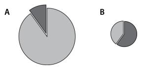
**Figure 17**. Creating wedge-shaped subsamples from cross-sectional disks from relatively large disks (A), and relatively small disks (B). In both A and B, the dark grey area is between 100-400g, and the light grey is discarded.
