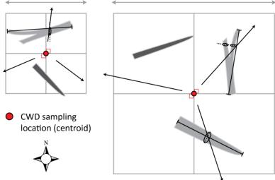
**Figure 2**. Illustration of three randomly oriented LIDS transects (arrow vectors) superimposed over a 20m x 20m plot (*left*), and a 40m x 40m plot (*right*). Transects start 3 m from the plot centroid (red circle). Light gray shapes are particles intersected by the CDW tally transects, and the black capped lines illustrate the central axis length of the particles. Darker gray shapes are CDW particles that do not intersect LIDS transects and are suitable for CDW bulk-density sampling.
