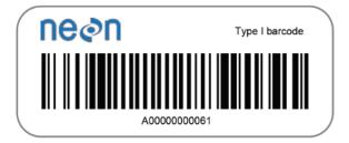
**Figure 8**. An example of a Type I barcode. These large-size, field-tolerant barcodes have a prefix of 'A' followed by 11 numbers.
